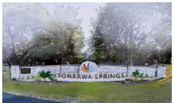
Option 2: “Slab” $27,000. Cut “Alamo” off wall. Re-cap. Set large stone slab in front of wall, mount splash logo to it. Mount 24” dimensional letters on concrete base in front.
