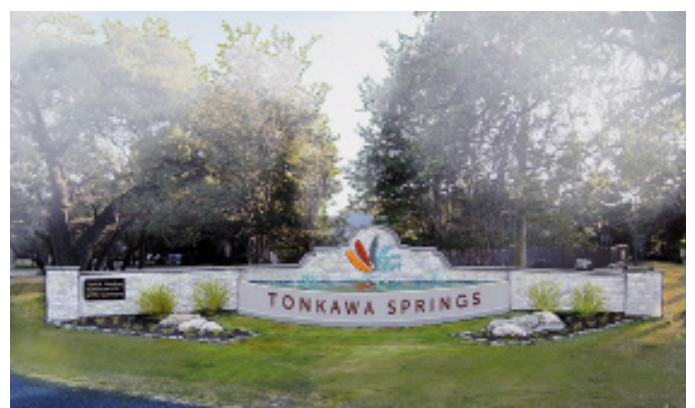
Option 3: “Planter/Water Feature” $30/37,500. Build 40” tall curved, concrete retaining wall to be a planter or water feature with fountains. Mount 20” metal letters on wall.
